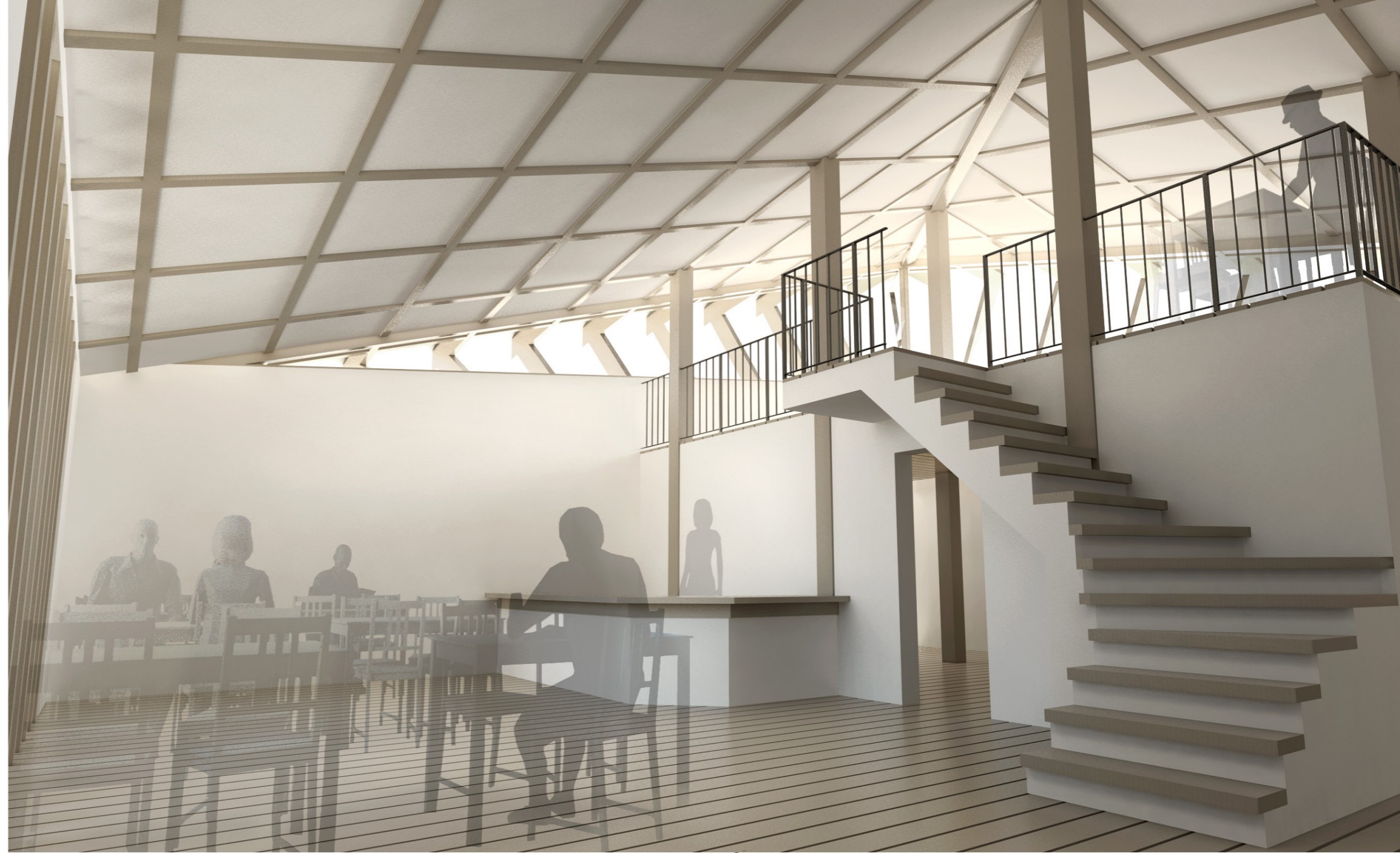
THE WOODEN CONSTRUCTION IS EXPOSED IN THE ENTRANCE AND RESTAURANT PART
